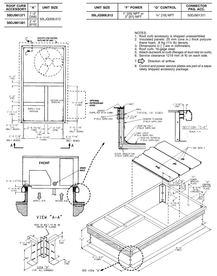
Fig. 1 — Roof Curb Dimensions
